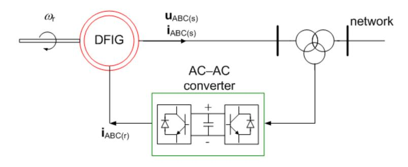
$\mathbf{u}_{ABC(s)}$  – 3-phase stator voltage,  $\mathbf{i}_{ABC(s)}$  – 3-phase stator current,  $\mathbf{i}_{ABC(r)}$  – 3-phase stator current,  $\omega_r$  – rotor angular velocity.
