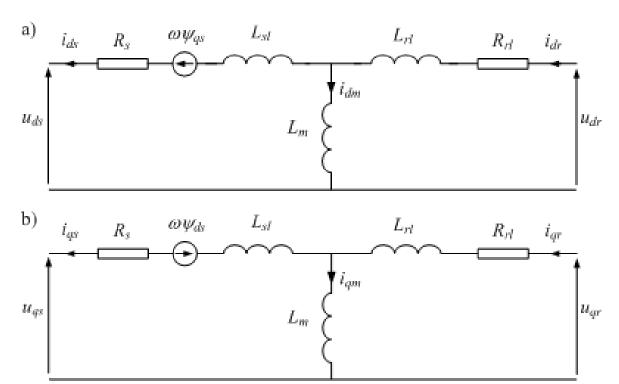
$$\underline{u}_{dq(s)} = -R_{s} \underline{i}_{dq(s)} - R_{r} \underline{i}_{dq(r)} - L_{sl} \frac{d}{dt} \underline{i}_{dq(s)} - L_{rl} \frac{d}{dt} \underline{i}_{dq(r)} - j\omega \left( L_{s} \underline{i}_{dq(s)} + L_{m} \underline{i}_{dq(r)} \right) + \underline{u}_{dq(r)}$$
